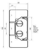
Compartments 1 & 3 = 1585mm² (each) total area Compartments 1 & 3 = 760mm² (each) 45% space factor Compartment 2 = 713mm² total area (with box) Compartment 2 = 342mm² 45% space factor (with box)
