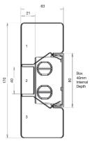
Compartments 1 & 3 = 2812mm² (each) total area Compartments 1 & 3 = 1265mm² (each) 45% space factor Compartment 2 = 760mm² total area (with box) Compartment 2 = 342mm² 45% space factor (with box)
